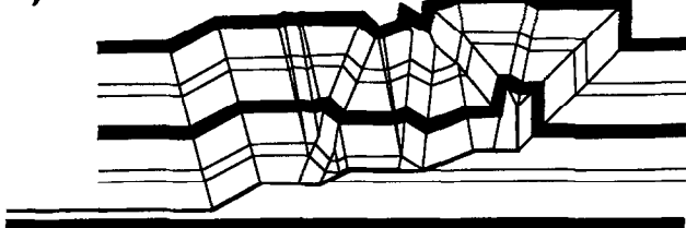
Fig. 13. Application of multibend, fault-bend fold theory to alternate fault terminations. (a) Wedge-thrusts, (b) fault-propagation folds, and (c) box folds can each be analyzed. Except for the fold termination itself, the fault system is treated as a fault-bend fold.
